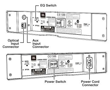
**EQ switch:** Use this switch to adjust the soundbar's bass for either wall or table mounting. If you're mounting the soundbar on a wall with the included wall-mount bracket, set the EQ switch to the "Wall" position for the most natural-sounding bass performance. If you are placing the soundbar on a table, set the EQ switch to the "Table" position for the most natural-sounding bass performance.
