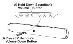
Press the TV remote's mute button while pressing and holding the soundbar's Volume + and Volume – buttons at the same time. If the programming was successful the soundbar's Surround button will change from amber to solid white for one second, then will return to flashing amber.
